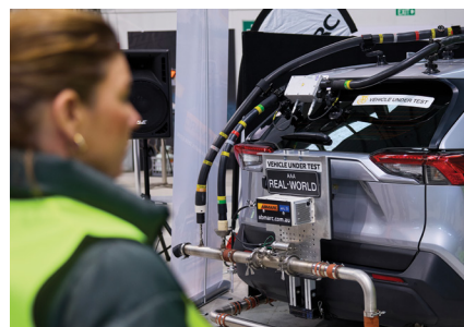
A RAV4 with emissions testing equipment.
