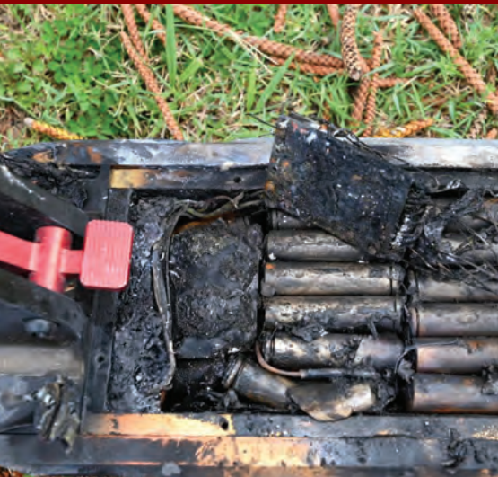
An e-scooter destroyed by a battery fire.
